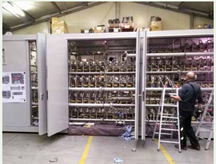
They work meticulously on the membrane container in parallel with the completion of the machine container. With the horizontal arrangement of the membrane modules, EnviTec is in a position to install more than double the number of modules in one single container.
